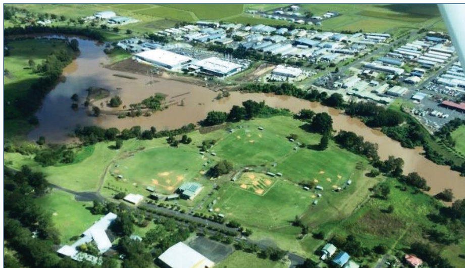
This picture of the floodway was taken on May 2 after heavy rainfall of more than 150 mm across the catchment. The gauge height at Lismore was about 7.2 metres AHD. The floodway starts flowing at 5.1 metres AHD.
