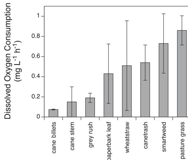
Figure 5. Mean ( $\pm$ SE,  $n = 3$ ) dissolved oxygen consumption rates by inundation of various dry vegetative materials at 20°C
