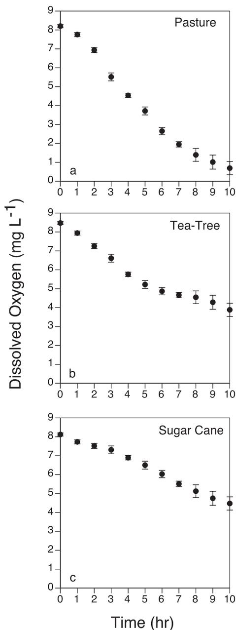
Figure 6. Mean ( $\pm$ SE,  $n = 3$ ) oxygen concentrations as a function of time in the *in situ* incubation experiments on three different land uses in the lower Richmond River catchment; (a) pasture, (b) tea tree and (c) sugarcane
