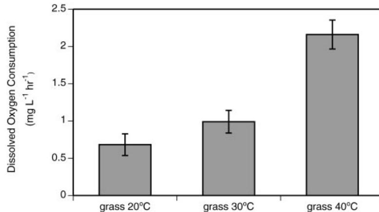
Figure 4. Mean ( $\pm$ SE,  $n = 3$ ) dissolved oxygen consumption rates by inundation of dry grass cuttings at three temperatures
