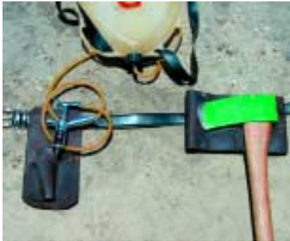
Stem injection can be conducted on foot using a 5 L backpack, injector gun and small axe.
