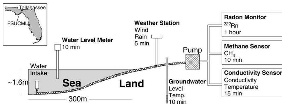
Fig. 1. Schematic representation of our monitoring system in FSUCML.
